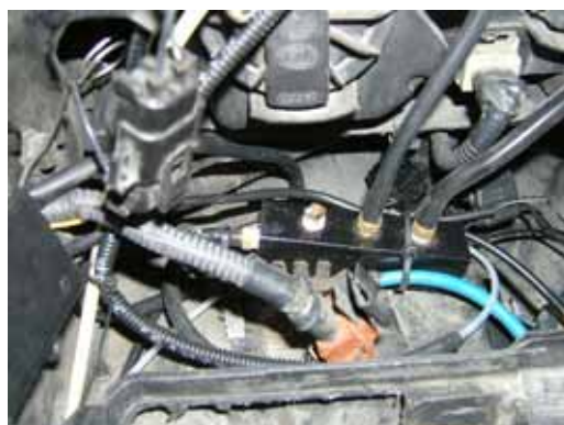
Here's a vacuum splitter that a buddy made for me. Not really necessary, but I like it more than using T splitters.
